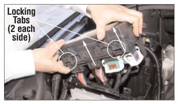
Locate fuse box in the engine compartment on the passenger side. Press the four (4) locking tabs (2 on each side) to disengage fuse box and lift up to expose empty compartment. Locking tabs may vary slightly from those shown above.
