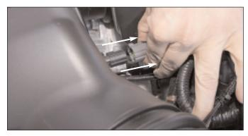
Disconnect the factory harness from the Intake air temp sensor.
