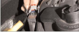
Disconnect the factory connector from the 3-Pin MAP sensor. This connector has a locking clip that must be slid back to unlock. Notice the slight difference in the position when the tab is in the "UNLOCKED" position. Then, squeeze down the locking tab, and push the connector in slightly (toward sensor) and then remove.
