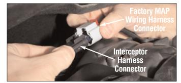
Plug the Interceptor harness connector into the factory MAP wiring harness connector, and push in the locking clip.
